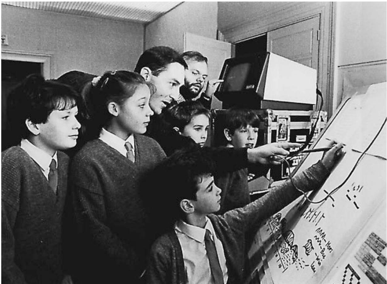
Figure 7.1 Music students composing with the UPIC system in 1983. Composer Iannis Xenakis conceived the UPIC system in the 1970s. The digital system for composition allowed users to draw notes and automation curves with a tablet and stylus interface. Today it is comparatively simple to digitize hand-drawn automation curves created with a tablet interface and use optical note recognition to recognize hand drawn notation on staff paper. Image from “Huddersfield Contemporary Music Festival Review” in the November 26, 1987 publication of the Huddersfield Daily Examiner (Bourotte and Delhaye).
